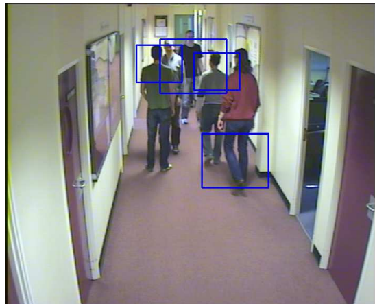
Figure 5.4: This shows a frame in a sequence showing the main head and shoulder detections. Note there are both true positive and false positive detections.
