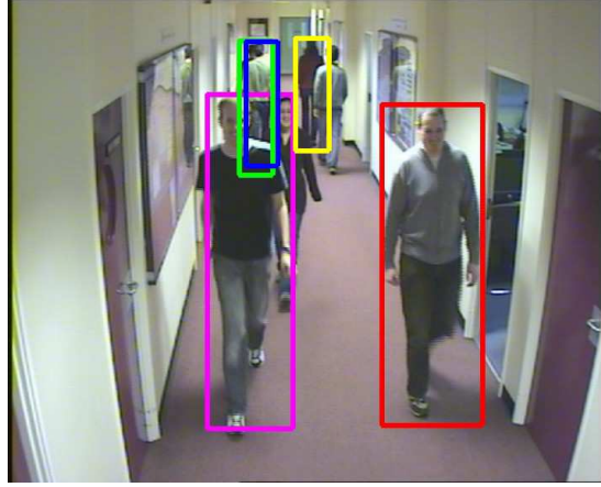
Figure 4.1: Objects detected by Connected Component Analysis on a image frame.
